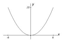
From this we find an equation for the parabolic shape. Since we placed the origin at the vertex of the parabola, we know the equation will have form  $y(x) = ax^2$ . Our equation will need to pass through the point (6,18), from which we can solve for the stretch factor a:
