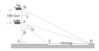
measure  $\gamma = 47^{\circ}$ . Determine the width of the clearing to the nearest foot. [UW]
